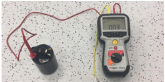
Figure 3 Test electrode with an insulation tester
