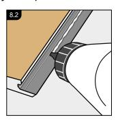
Where the planks can no longer be installed together using the Angled Fold Down Installation method. Remove the upstand on the locking element of the protruding lower female profile (fig. 8.1). Then, use a suitable contact adhesive in accordance with the manufacturer's instruction (fig. 8.2) to connect the planks. Remember to place spacers between these planks and the wall to maintain the expansion gap.
