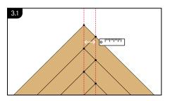
Measure the distance between the two straight lines, originating from the corners of the planks.
