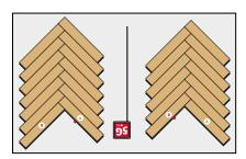
When a plank is correctly locked, it may not be possible to take it up or remove it by hand without damaging the planks. Planks can be dismantled using a 0.9mm wire.
