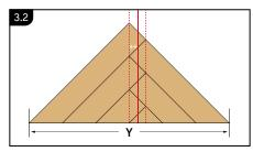
Divide this number by two and get the X measurement. The Y measurement is the width of the triangle at its widest point as show in figure 3.2.
