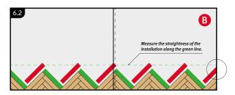
Next install the B-planks. Cut in the last piece on the right hand side (as indicated) to fit to the perimeter wall, not forgetting the expansion gap. Measure the alignment of the tips of the triangles along the horizontal dotted green line above using a suitable length straight edge. Repeat this check throughout the remainder of the installation. Any deviations should be brought back in line.
