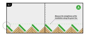
Install A-planks to connect the triangles. The joints need to be checked carefully to ensure the planks are correctly aligned and fully engaged. Cut in the last piece on the left hand side (as indicated) to fit to the perimeter wall, not forgetting the expansion gap.
