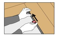
Align the 0.9mm wire with the installed 5G joint so that the wire is between the profile of the last installed plank and the flexible tongue. Push forward the 0.9mm wire into the joint. This pushes back the flexible tongue and releases the plank for dismantling.
