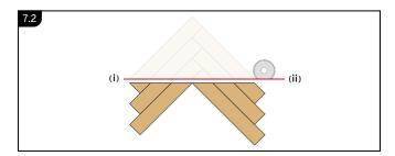
Carefully remove spacers to complete the installation.
