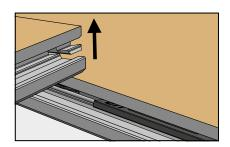
The plank should now lift up easily on the long side.
