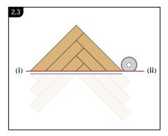
Using a plunge/circular saw set at the correct depth – cut the assembled triangle at the marked line from point (i) to (ii). Alternatively, the marked triangle can be disengaged and cut with a utility knife, prior to reassembling the triangle.
