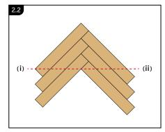
Install the planks precisely and in the order indicated by the numbers on the planks in figure 2.1. Carefully check that each individual plank is correctly aligned and engaged. Mark a line from points (i) to (ii) as illustrated in figure 2.2, ensuring that a 45 degree angle is achieved.
